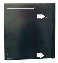
7. Slide the outer cover back about 1 inch toward the rear of the oven. Lift the cover from the oven.
