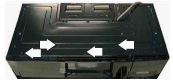
3. Remove 5 Phillips-head screws from the back of the oven.
