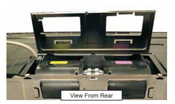
4. Lift out the vent blower and place it on top of the oven side as shown below and disconnect the electrical connector to the vent blower.
