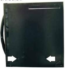
6. Remove 2 Phillips-head screws from the left side of the oven.
