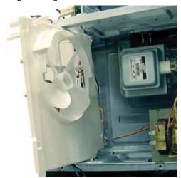
8. Using a small flat blade screwdriver, carefully remove the fan retainer.
