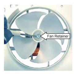
9. Remove 2 Phillips-head screws that attach the fan motor to the cooling fan frame.
