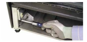
7. Remove the five 1/4-in. hex-head screws (3 at the rear and 2 on top) that attach the rear vent to the range. Lift and remove the rear vent.
