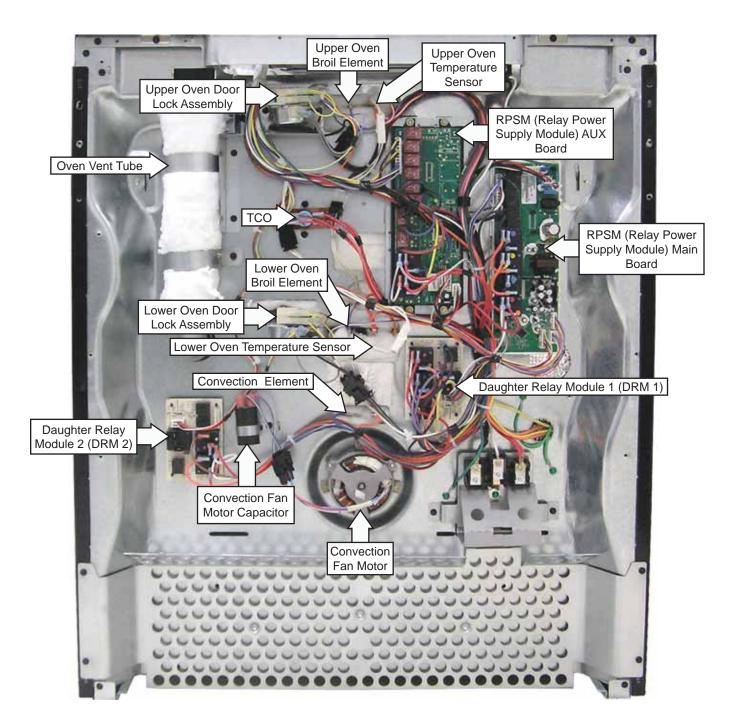
Note: The upper and lower oven bake element terminals are located behind the left side panel.
