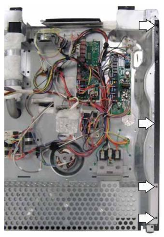
9. Remove the three 1/4-in hex-head screws from the top of the side panel.
