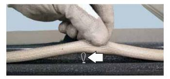
On PHS925, the bottom center clip joins both ends of the gasket to form a continuous seal. Make sure this clip is inserted into the bottom center hole in the inner door panel.
