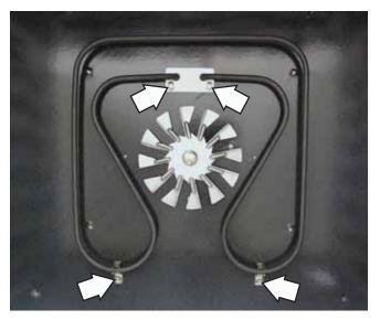
3. Carefully pull the convection element towards the front of the oven until the element terminals are accessible.
