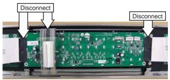
3. Remove the two 1/4-in. hex-head screws that attach the right side of the main logic board to the control panel.
