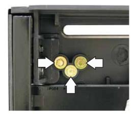
6. Remove four 1/4-in. hex-head screws that attach each side brace to the outer door panel.
