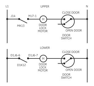
The display will flash "DOOR  $\square$ " if the lock switches are not set to satisfy present lock or unlock request. The motor relay will be energized.
