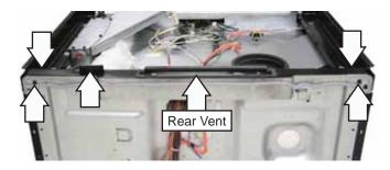
8. Remove the three 1/4-in hex-head screws from the top front of the control panel support.
