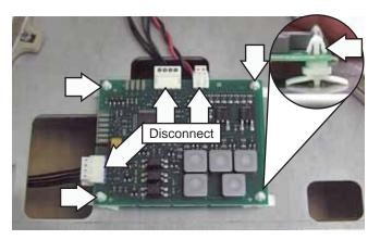
**Note:** The hot surface indicator LEDs are located on the bridge board. The LED will be turned on when the cooktop element is turned on and will remain on as long as the glass temperature exceeds 150°F.
