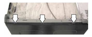
**Note:** The front of the panel is held to the range frame by 3 plastic grommets that engage 3 keyhole slots placed along the inside front flange of the panel.
