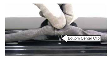
On PS978, make sure the gasket is cross tucked in the bottom slots of the inner door panel. Use a small screwdriver to tuck the loose ends of the gasket into the slots. The overlap is required to ensure a proper door seal.
