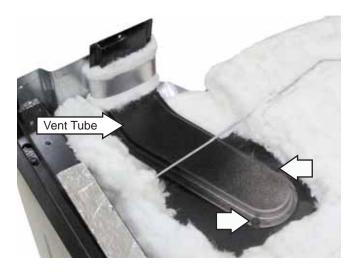
6. Grasp and carefully remove the vent tube from under the rear wire insulation retainer.
