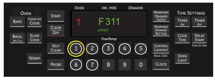
The F-Code log can be erased by pressing 9 and 0 together while the log is being displayed.
