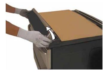
4. Disconnect the 2 (PHS925) or 3 (PS978) range wire harnesses from the main logic board and place the control panel face down on the protective surface.
