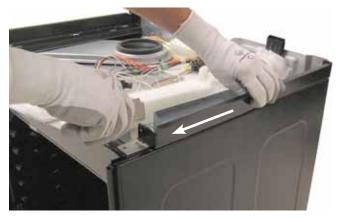
14. Remove the two 1/4-in hex-head screws from the back of the side panel.
