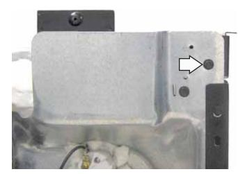
7. Carefully lift the left side of the control panel support, slide the extension brace forward, and remove the extension brace from the range.
