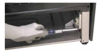
7. Remove the five 1/4-in. hex-head screws (3 at the rear and 2 on top) that attach the rear vent to the range. Lift and remove the rear vent.
