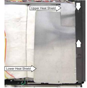
9. Remove the 1/4-in. hex-head screw from the back of the top brace.
