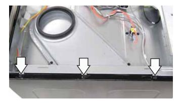
**Note:** The front of the panel is held to the range frame by 3 plastic grommets that engage 3 keyhole slots placed along the inside front flange of the panel.
