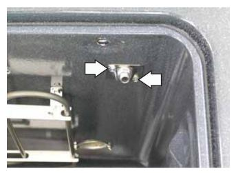
After removing the two 1/4-in. hex-head screws, the outlet and wiring can then be pulled down from the oven wall approximately 3 inches.
