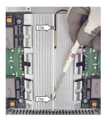
3. Mark the location of the black L1 and the blue L2 wires and disconnect both from the generator board.
