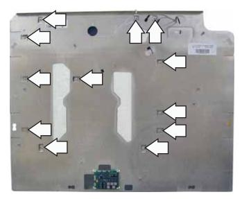
6. Lift the front of the aluminum plate up and disconnect the ground wire.
