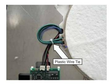
7. Lift and fold back the insulation from the wire entry in the aluminum plate.
