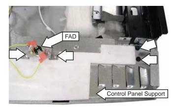
11. Remove the two 1/4-in. hex-head screws from the extension brace.
