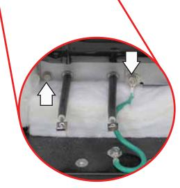
20. Using a small flat blade screwdriver, pry the left side of the retainer away from the element.
