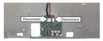
4. Fold back insulation and place the filter-tobridge board and cooling fan harnesses inside the module.
