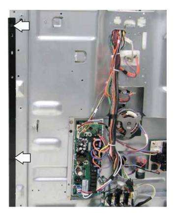
15. Remove the three 1/4-in hex-head screws from the top of the side panel.
