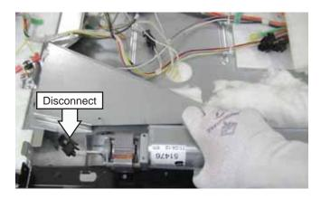
The FAD is a low voltage thermal switch. It is attached with two 1/4-in. hex-head screws to a bracket that is attached to the control panel support. The FAD disconnects the common (yellow) of the lock logic circuit when the control compartment area gets too hot or the cooling fan fails. The FAD will open at 230°F and is resetable. The FAD is active during all operations.
