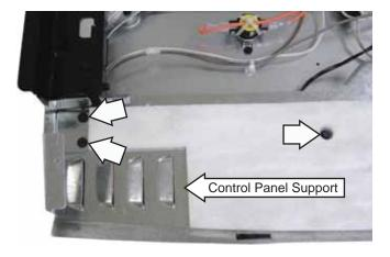
9. Remove the three 1/4-in. hex-head screws from the extension brace.
