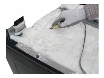
5. Remove the 2 hex-head screws that attach the vent tube to the top of the oven liner.
