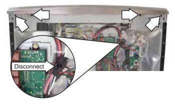
6. Remove the eight 1/4-in. hex-head screws from the rear vent. Lift and remove the rear vent.
