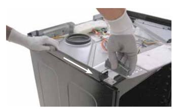
13. Remove the three 1/4-in hex-head screws from the top of the side panel.
