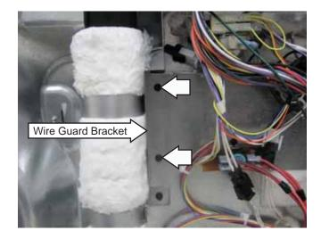
4. Disconnect the light assembly wire harness.
