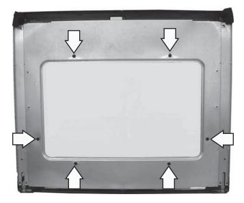
5. Remove the insulation and the inner glass assembly from the inner door.
