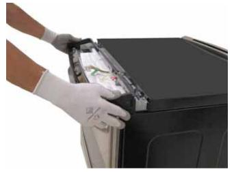
5. Remove the four 1/4-in. hex-head screws (2 on each side) that attach the front of the cooktop frame to the range.
