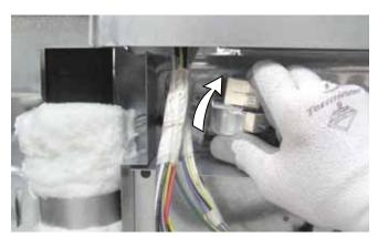
8. Remove the door switch wire retainer from the top of the mounting plate, and then pull the lock assembly out from the range.
