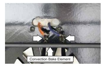
4. Disconnect the wires from the convection element.
