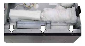
**Note:** The front of the panel is held to the range frame by 3 plastic grommets that engage 3 keyhole slots placed along the inside front flange of the panel.
