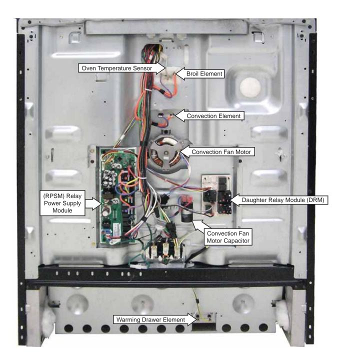
Note: The oven bake element terminals are located behind the left side panel.
