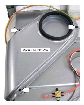
12. Lift and separate the induction module air inlet vent from the air tunnel and unhook the bottom of the air tunnel from the range frame.
