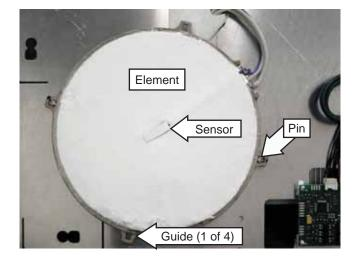
Note: Replacing the 11-in. element will require cutting off and replacing the plastic wire tie joining bridge board wiring and element wiring.
