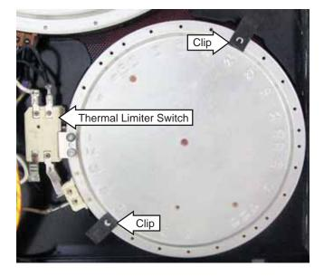
Note: When installing a radiant element, make sure the element is firmly pressed against the glass and aligned in the target area.
