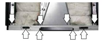
7. Remove the four 1/4-in. hex-head screws that attach the blower assembly to the rear vent.
