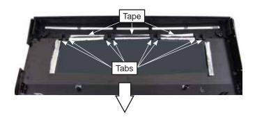
To replace the inner door assembly of the upper oven door on PS978:
