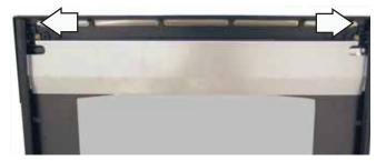
Note: When installing the door handle, make sure the handle is level with the top of the door before attaching the heat deflector. An enlarged hole for the right side screw has been provided for this adjustment.
