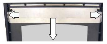
4. Remove the two 1/4-in. hex-head screws that attach the handle and top trim.
