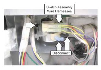
7. Grasp the rear of the lock assembly. Lift and rotate it approximately 40 degrees clockwise and pull it out approximately 2 inches.
