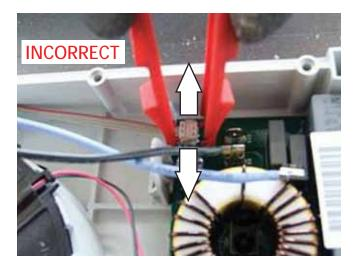
**Correct way**: Use side-to-side motion to remove the LINbus connector.
