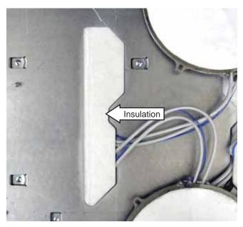
8. Note the routing of the element wires, and loosen the 2 slotted T-25 Torx screws holding the element wires to the generator board.
