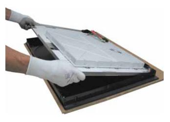
Note: When installing the aluminum plate to the cooktop, be sure to install spacers with the shoulder toward cooktop.
