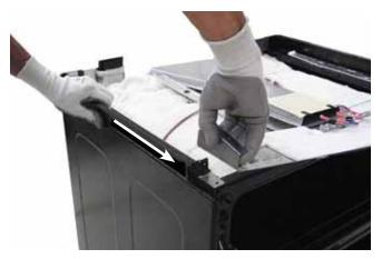
8. Remove the four 1/4-in hex-head screws from the back of the side panel.
