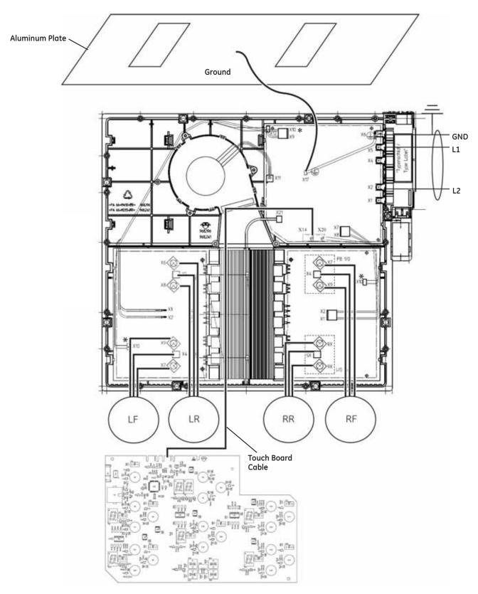
Caution: \*A special tool is required when removing the connections (marked with an \*) from the circuit boards. (See *LINbus Connectors*.)
