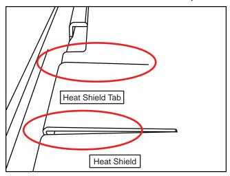
To correct a misaligned heat shield it is necessary to remove the glass top. (See *Glass Top.*)
