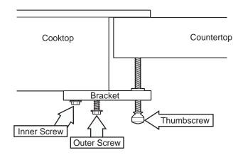
4. Turn the bracket inwards to avoid interference when lifting the cooktop from the countertop.
