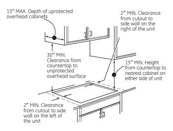
If a 30-in. clearance between the cooking surface and overhead combustible materials or metal cabinets cannot be maintained, a minimum clearance of 24-in. is required and the underside of the cabinets above the cooktop must be protected with not less than 1/4-in. insulating millboard covered with sheet metal not less than 0.0122-in. thick.
