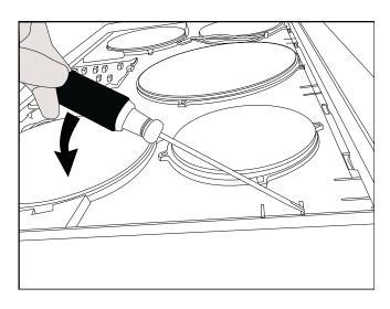
Inspect all tab-to-heat shield alignment areas. Repeat this alignment procedure on all tabs, if necessary.
