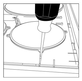
The heat shield can be aligned with the tab by pushing down on the screwdriver and raising the heat shield even with the tab.
