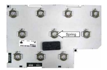
**Note:** If one or more functions do not work and no apparent damage is present, the cause can be an excessive flat-bottom drop of the packaged unit during shipping/handling. The force of the drop can position the heat shield out of proper alignment to the heat shield mounting tabs. This would cause improper spacing between the underside of the glass top and the capacitive switches on the module, rendering the switches inoperative.
