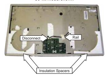
5. On 36-in. models, remove the fourteen 1/4-in. hex-head screws, (5 on the front, 5 on the back, and 2 on each side) from the outside of the burner box. (On 30-in models, remove the 10 1/4-in. hex-head screws, (3 in the front, 3 in the back, and 2 on each side) from the outside of the burner box.)
