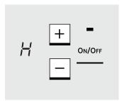
"H" indicates that the Boost power level has been selected for rapid cooking and boiling.
