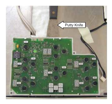
**Note:** Make sure all springs and capacitance foam pads are in place for precise touch sensitivity between the touch board and the cooktop glass.
