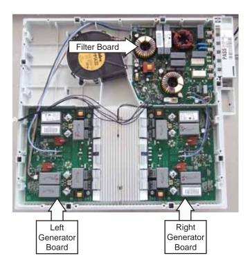
Generator board maximum output is 3700W. When using an element on high and a second element sharing the same generator board is then operated, the second element will receive priority. For example, if the first element was using 3700W when the second element was turned on, power on the first element will be reduced to a lower setting.
