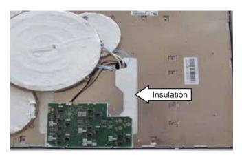
5. Note the routing of the element wires and loosen the two slotted T-25 Torx screws holding the element wires to the generator board.
