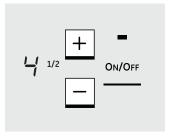
The power level with a fraction indicates the additional half-step setting.
