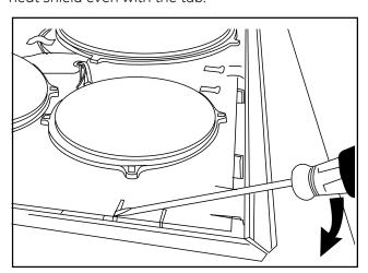
It may be necessary to insert the screwdriver in the right-side gap, push down on the screwdriver, and raise the heat shield even with the tab.
