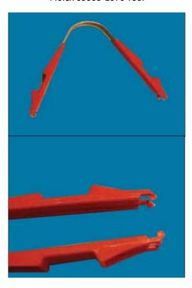
Do not use front-to-back motion to remove LINbus connector.
