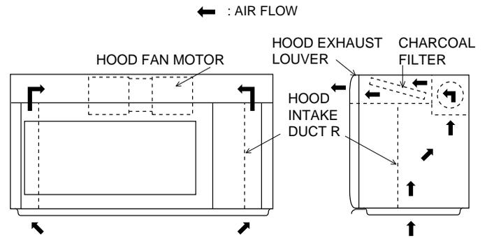
**VENTILATION METHODS HOT AIR EXHAUST**
