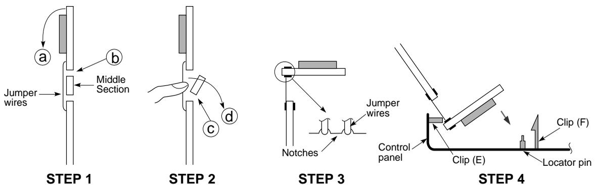
**POSITIVE LOCK® CONNECTOR (NO-CASE TYPE) REMOVAL**
