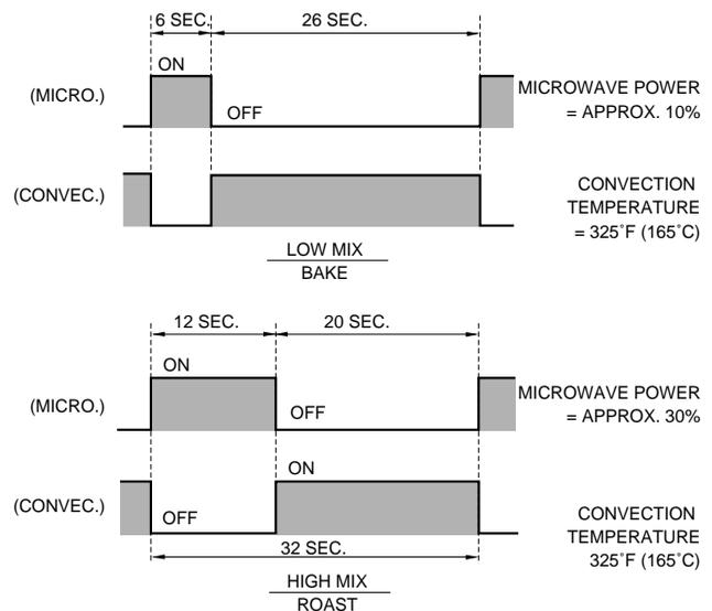
Note: During alternate Microwave/Convection operation, the convection heater is energized only if the cavity temperature drops below the set temperature.
