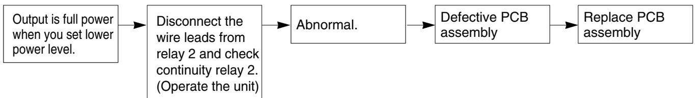
**(TROUBLE 6) When Microwave oven operates, strange cook can be seen on the display and stop with beep sound.**
