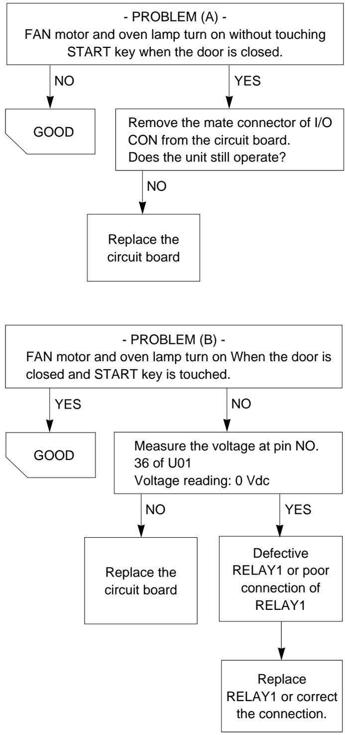
(3) CHECKOUT PROCEDURES FOR CIRCUIT BOARD
