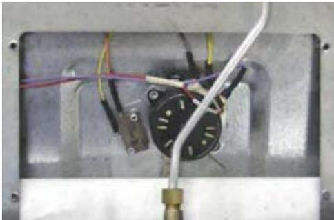
6. Mark and disconnect the wiring from the latch assembly.
