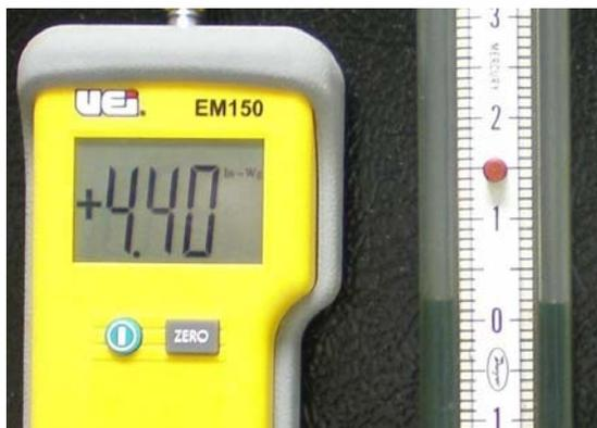
A manometer is essential for proper regulation of gas pressure and diagnosis of supply and combustion problems. You can use either a digital manometer or the older style slack-tube manometer.
