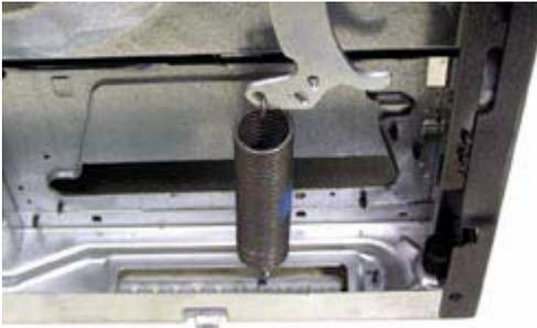
1. Remove the range from its installation.
