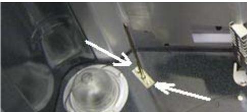
4. Remove the two ¼" hex head screws that attach the sensor to the oven wall.
