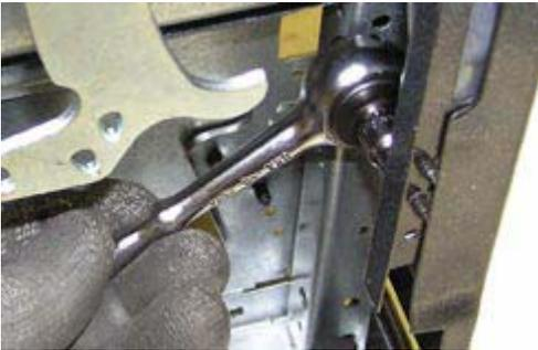
7. Remove the two  $\frac{1}{4}$ " hex head screws that attach the hinge to the frame.
