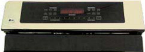
2. From the front, remove the two T-15 Torx® screws that attach the bottom of the control panel to the back guard.
