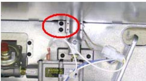
7. Remove the two hex head screws, located behind the warming drawer, that hold the burner in place and then remove the burner.
