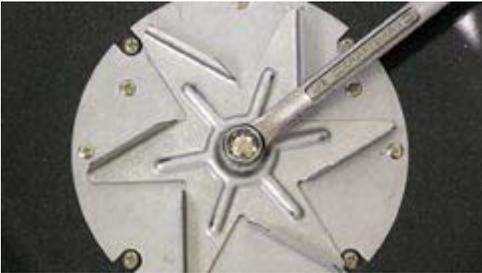
3. Use a 1/2" wrench to remove the nut from the convection fan blade. Hold the blade securely and turn the nut clockwise.
