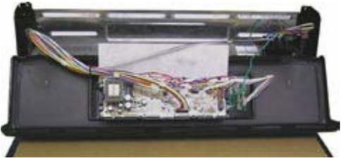
4. Carefully fold the control panel over the grates into the service position.
