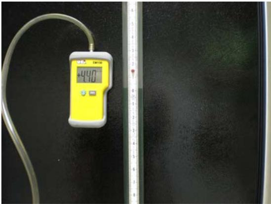
To measure the gas pressure, you'll need either a digital or water (slack tube) manometer.
