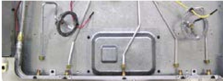
7. Remove the five burner valves from the gas manifold.
