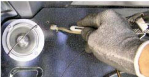
**NOTE!** When replacing the oven temperature sensor, the connector end must be positioned OUTSIDE the range insulation. The insulation should be allowed to fill around the lead wires to protect the sensor from any heat loss at the opening.
