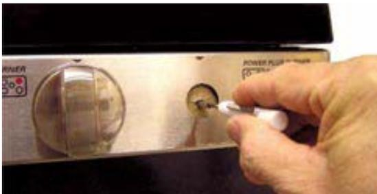
Remove the surface control knob and locate the adjustment screw in the center of the control valve shaft. A thin flat-blade screwdriver, approximately  $\frac{3}{32}$ " across, is needed to access the screw. Turn the adjustment screw until the flame reaches the desired size.
