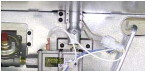
5. Disconnect the ignitor wires located behind the warming drawer. Gently pull the connector through the oven floor and remove the ignitor.
