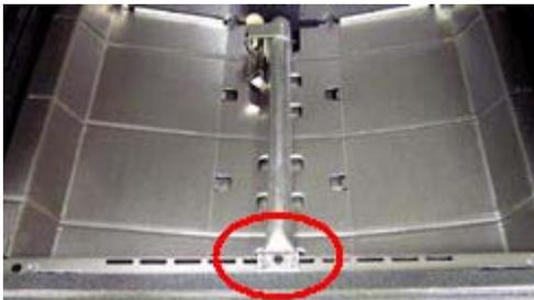
6. Remove the hex head screw that holds the front of the burner in place.
