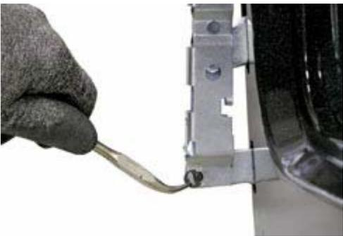
6. Remove the E-clips from the hinge pin and remove the pin.
