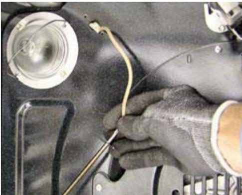
5. Gently pull the sensor wire in to the oven cavity.
