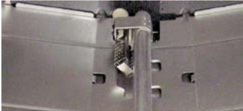
4. Remove the two hex head screws that hold the ignitor to the bake burner.
