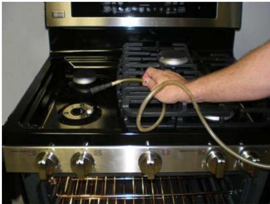
Measuring gas pressure can be easily accomplished at any of the 5 surface burners.
