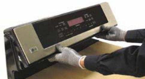
3. Grasp and pull the bottom of the control panel out about one inch and lift it off the top rear corner screws.
