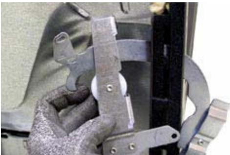
8. Position the top of the hinge body into the notch in the hinge arm (see photo) and rotate the hinge body clockwise to remove.
