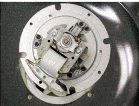
6. Disconnect the 3-wire connector from the motor.
