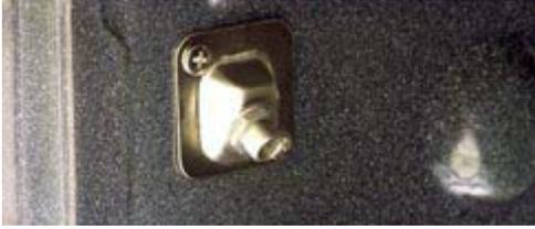
1. Remove the two Phillips screws that attach the probe outlet to the oven.
