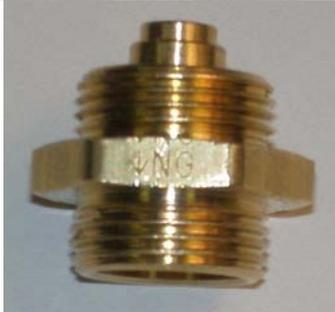
Note the marking that shows the short end to be installed for natural gas. On the other side, the arrow points toward the longer end for propane (LP).
