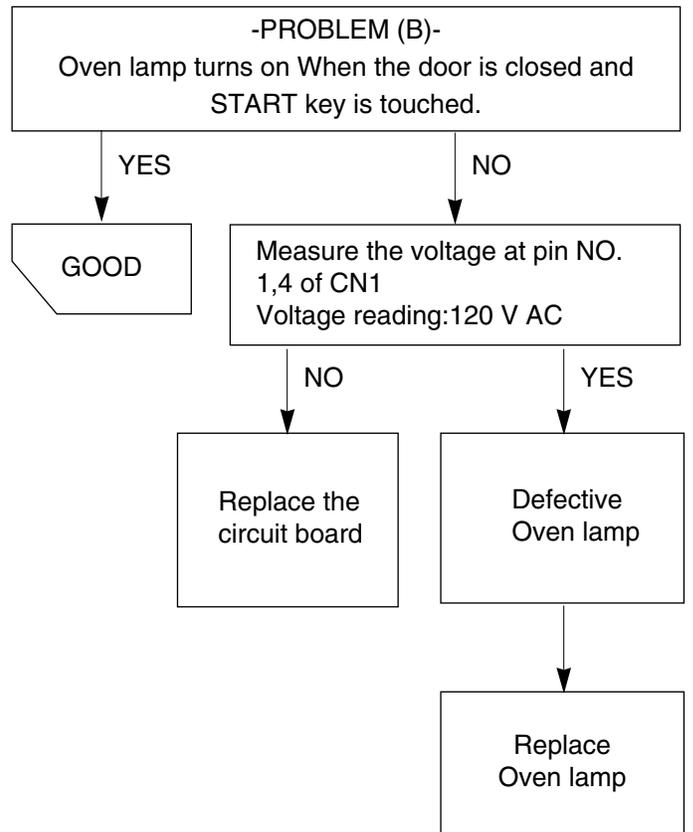
(3) CHECKOUT PROCEDURES FOR CIRCUIT BOARD
