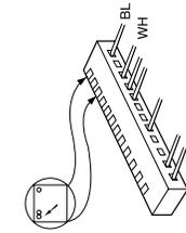
Measure voltage between pin 1 and pin 3 of connector CN1.
