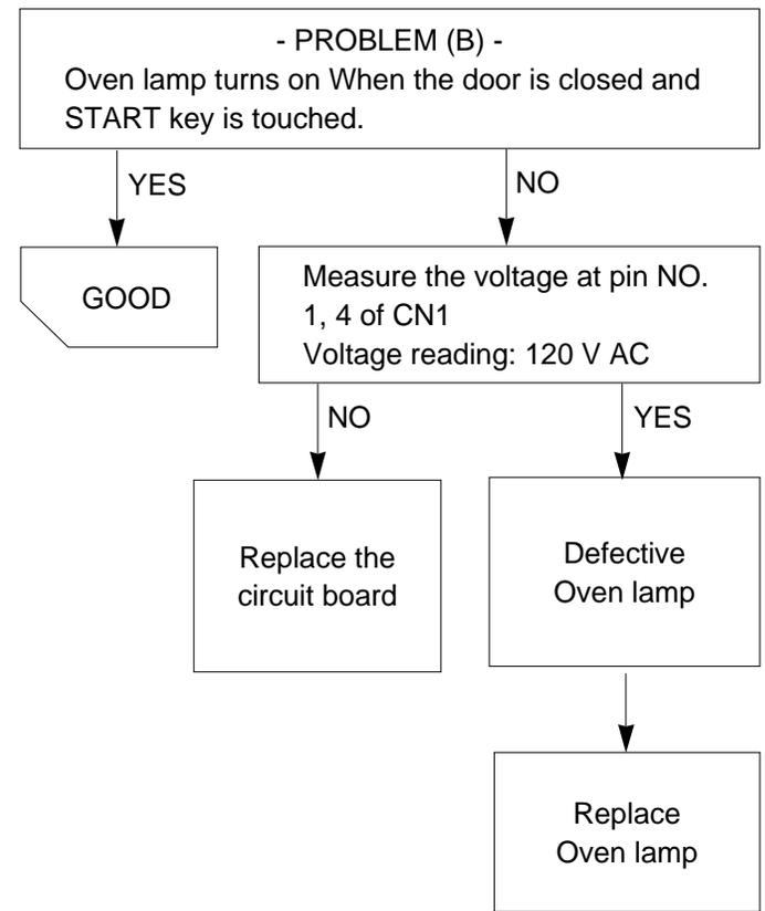
(3) CHECKOUT PROCEDURES FOR CIRCUIT BOARD
