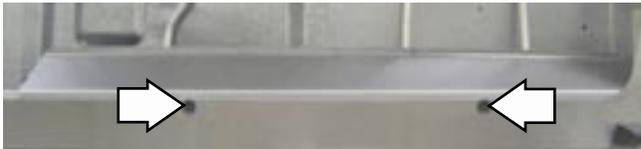
4. Remove the four ¼-in. hex-head screws that hold the latch assembly cover in place. Remove the cover.
