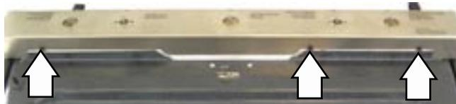
8. Pull the manifold panel straight out from the range.
