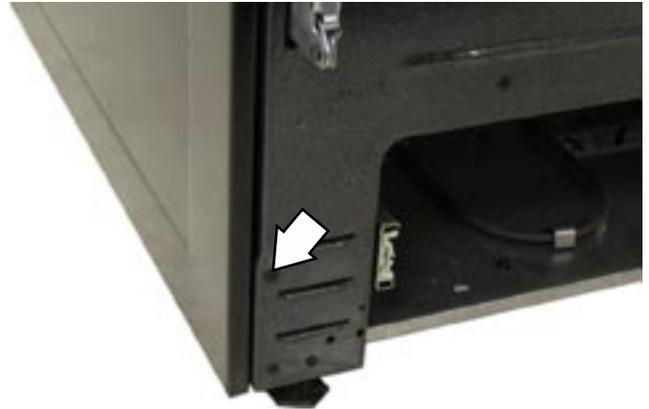
7. Remove four 1/4-in. hex-head screws from the back edge of the side panel.
