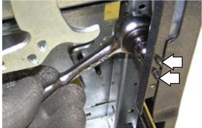
8. Position the top front of the hinge body into the notch in the hinge arm (see photo) and rotate the hinge body clockwise to remove.
