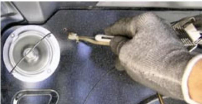
**IMPORTANT:** When reinstalling the oven temperature sensor, the connector end must be positioned **OUTSIDE** the range insulation. Insulation should be allowed to close in around the oven temperature sensor lead wires thus protecting the sensor from any heat loss at the insulation opening.
