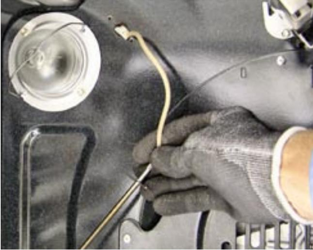
**Note:** When reinstalling the sensor, use a small flat-blade screwdriver to push and guide the sensor wire harness into the oven liner.
