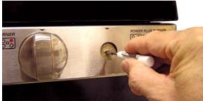
**Note:** Low setting adjustments must be made with 2 other burners in operation on a medium setting. This procedure prevents the low flame from being set too low, resulting in the flame being extinguished when other burners are turned on.
