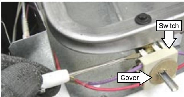
**Note:** When replacing an ignitor switch, cut the switch wires and splice the new switch using approved connectors and heat shrink tubing.
