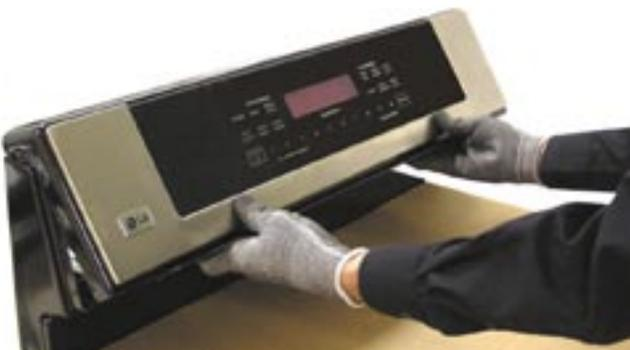
5. Carefully support and position the control panel on the burner grates in the service position.
