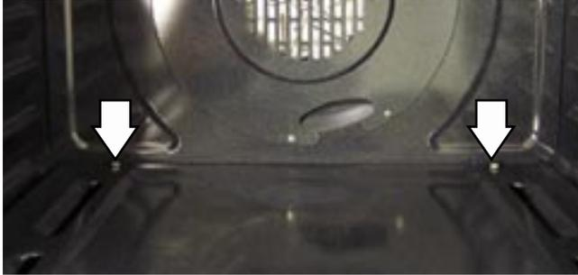
4. Remove the 2 hex-head screws that hold the glow-bar igniter to the bake burner.
