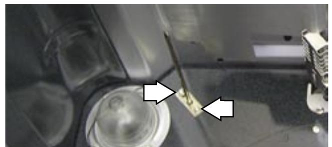
6. Gently pull the sensor wire harness into the oven.
