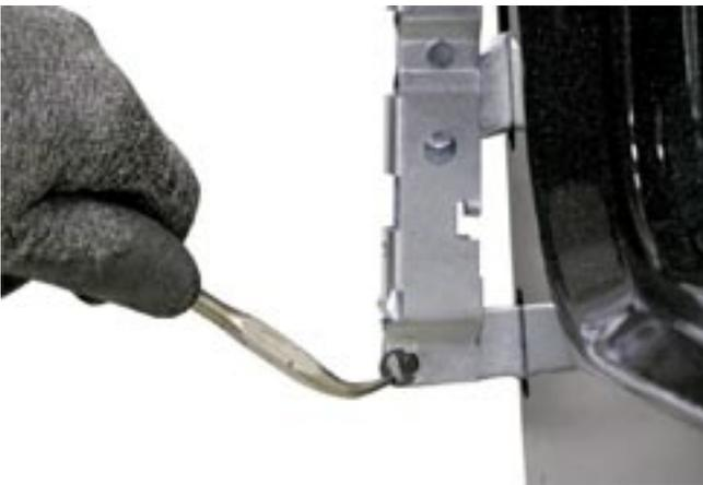
7. Remove the two 1/4-in. hex-head screws that attach the hinge to the frame.
