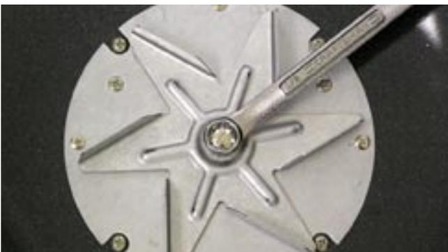
4. Remove the fan blade and washer from the fan motor shaft.
