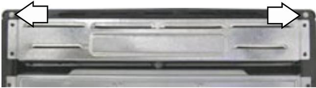
3. Remove the two T-15 Torx screws that attach the bottom of the control panel to the backguard.
