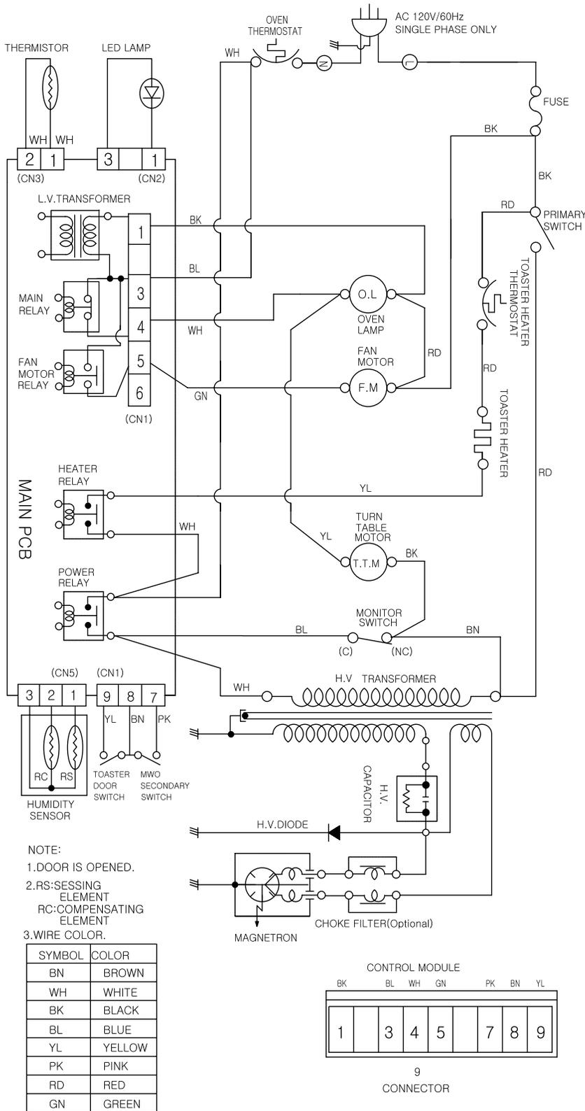
IMPORTANT SAFETY NOTE: THE SHADED AREAS ON THIS SCHEMATIC DIAGRAM INCORPORATE SPECIAL FEATURES IMPORTANT FOR PROTECTION FROM MICROWAVE RADIATION, FIRE, ELECTRICAL SHOCK, AND HAZARDS. WHEN SERVICING IT IS ESSENTIAL THAT ONLY MANUFACTURER'S SPECIFIED PARTS BE USED FOR THE CRITICAL COMPONENTS IN THE SHADED AREAS OF THE SCHEMATIC DIAGRAM.
