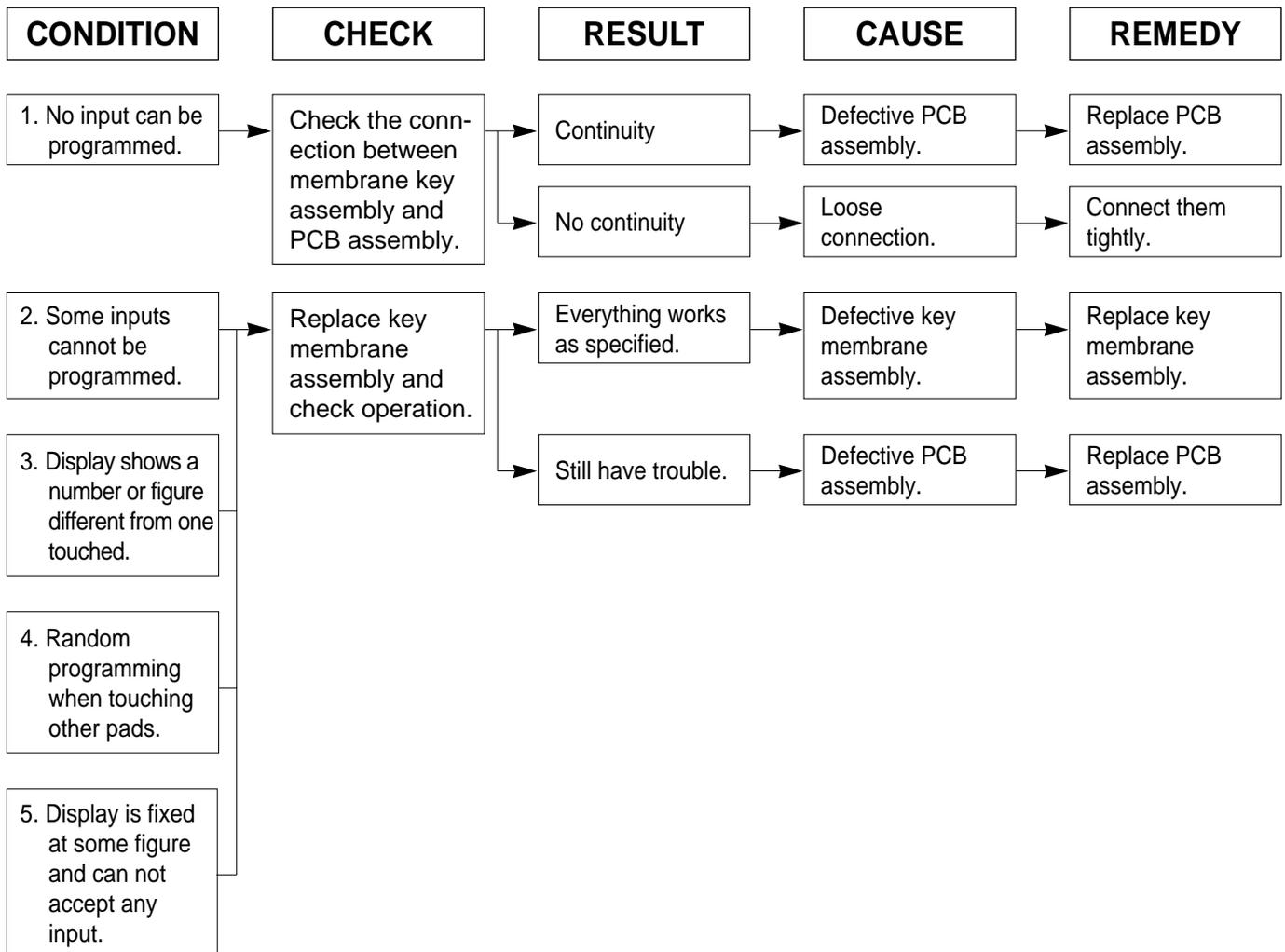
**(TROUBLE 2) Oven does not operate at all, display window does not display any figures, and no input is accepted.**
