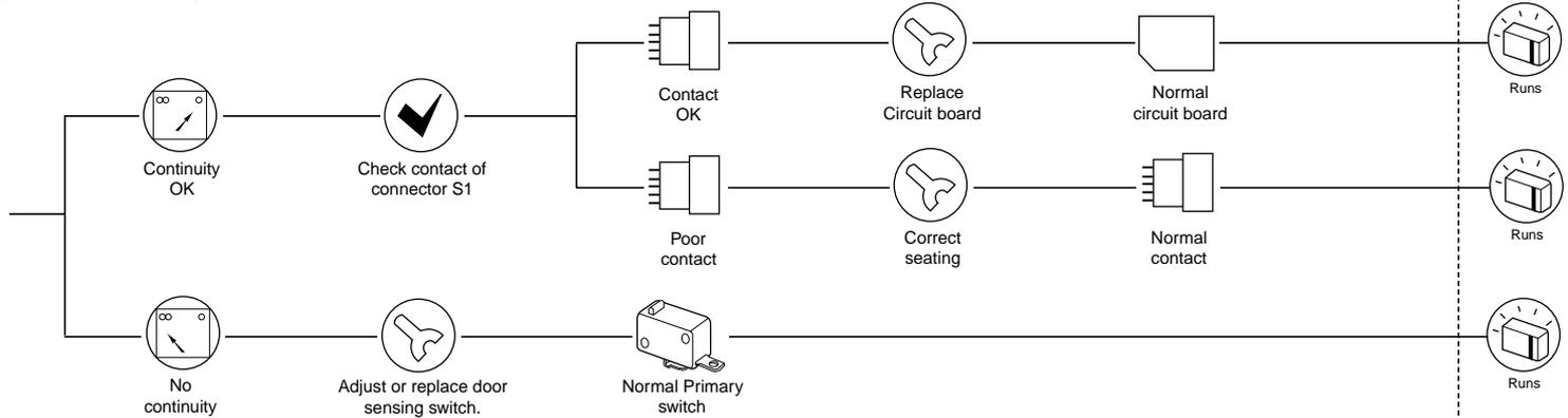
**PROBLEM - D:** Unit operation seems to be normal but little or no heating is produced in oven load.
