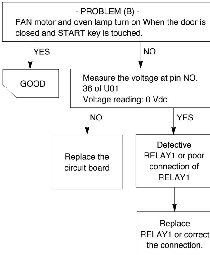
(3) CHECKOUT PROCEDURES FOR CIRCUIT BOARD
