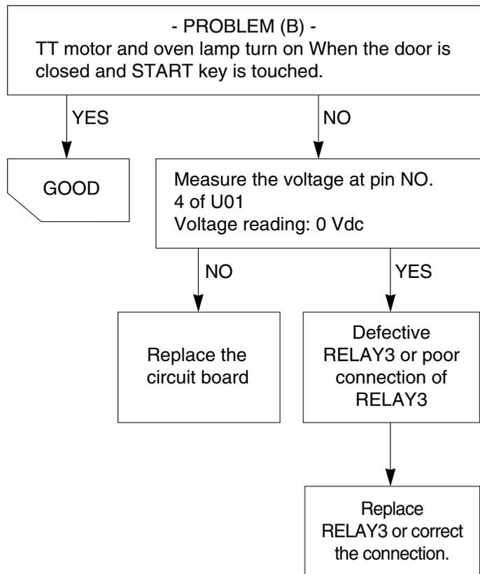
(3) CHECKOUT PROCEDURES FOR CIRCUIT BOARD
