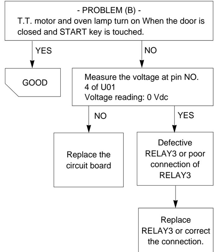
(3) CHECKOUT PROCEDURES FOR CIRCUIT BOARD
