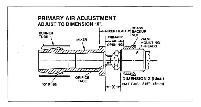
Primary air adjustments are pre-set at the factory. No further adjustment should be needed. If for any reason it should become necessary to make primary air adjustments, follow the procedure below.
