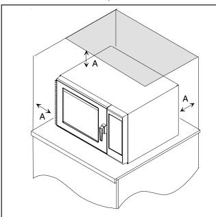
A—Allow at least 1½ inches / 3.81 centimeters of clearance around top and sides of equipment. Proper air flow around equipment cools electrical components. With restricted air flow, oven may not operate properly and life of electrical parts is reduced.
