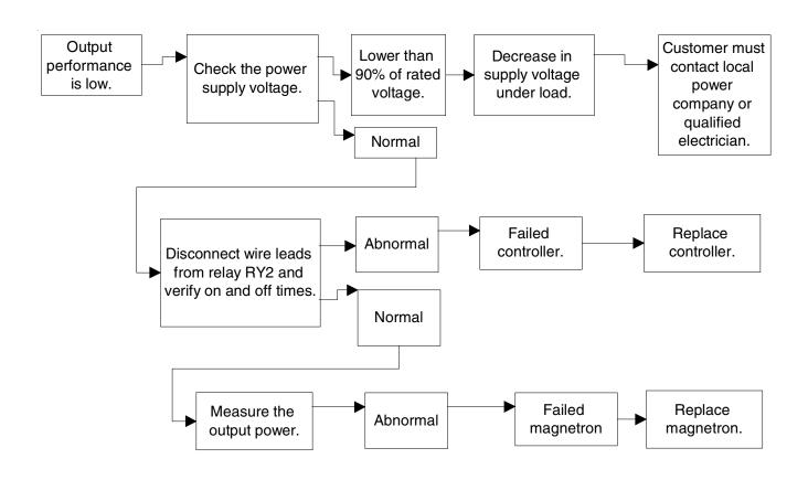
**NOTE:** Simple test of power output can be conducted by heating one liter of water for one minute. Refer to Power Test on page 24 of this manual.
