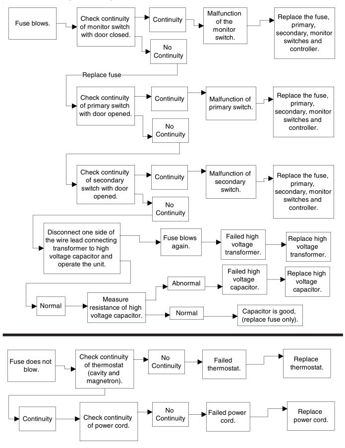
Trouble 3: Display shows all digits programmed, but does not start cooking when the START pad is pressed.
