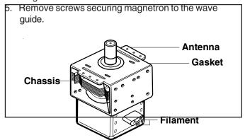
6. Replace magnetron and reverse procedure to reassemble.
