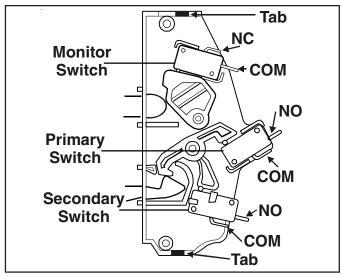
**NOTE:** After repairing the door or the interlock system, it is necessary to check the switch continuity before operating the oven.
