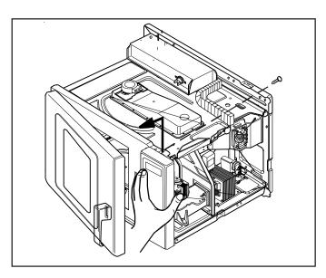
5. Replace component and reverse procedure to reassemble.
