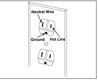
**NOTE:** Circuit tester can be used to verify voltage at outlet. Connect one lead to hot line and the other lead to ground. Circuit tester should light.
