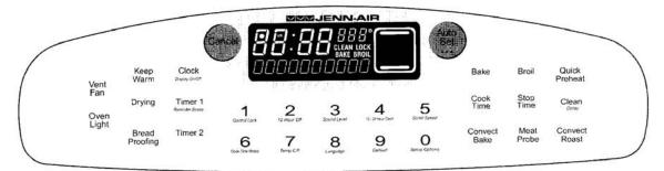
The electronic control is designed for ease in programming. The display window on the control shows time of day, timer and oven functions.
