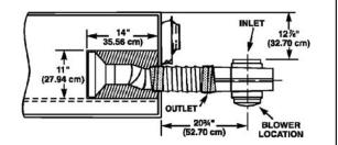
Figure 14 Left Cabinet (Top View)
