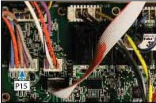
When the door is required to lock or unlock, the K3 relay energizes and sends line voltage to the door lock motor.
