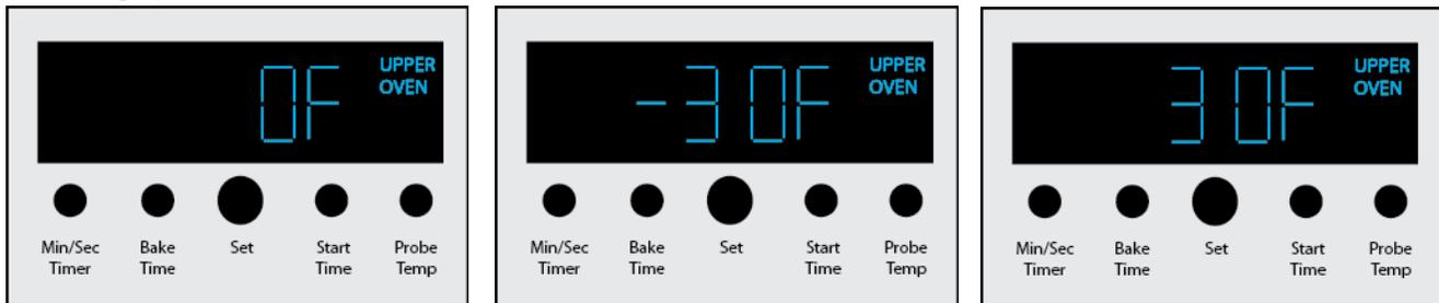
Once the proper adjustment has been made, depress “MIN/SEC TIMER” to accept the change. Then, depress “PROBE TEMP” to exit the Settings mode.
