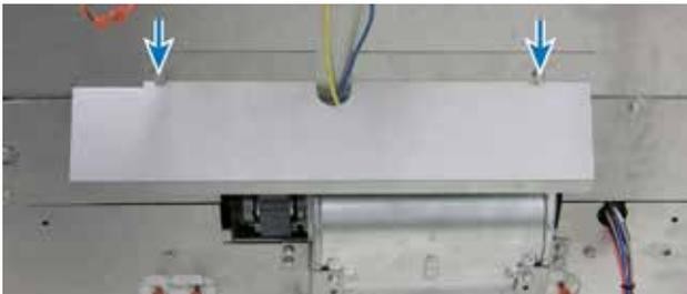
4. Remove screws securing cooling fan.
