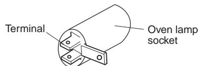
Figure C-1. Oven lamp socket
