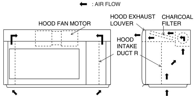
**VENTILATION METHODS HOT AIR EXHAUST**
