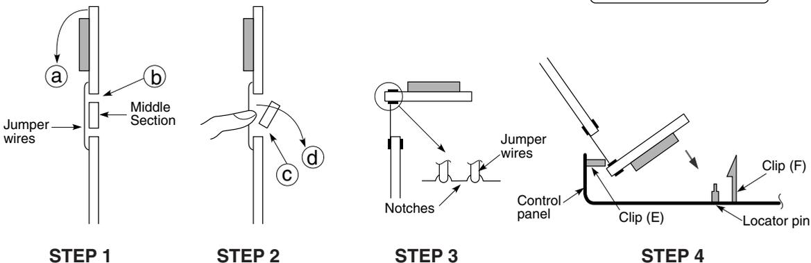
**POSITIVE LOCK® CONNECTOR (NO-CASE TYPE) REMOVAL**
