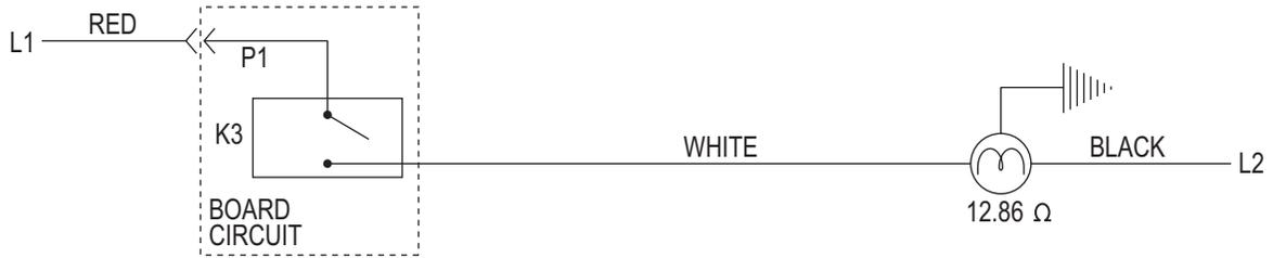
*Door Latch Motor Strip Circuit*
