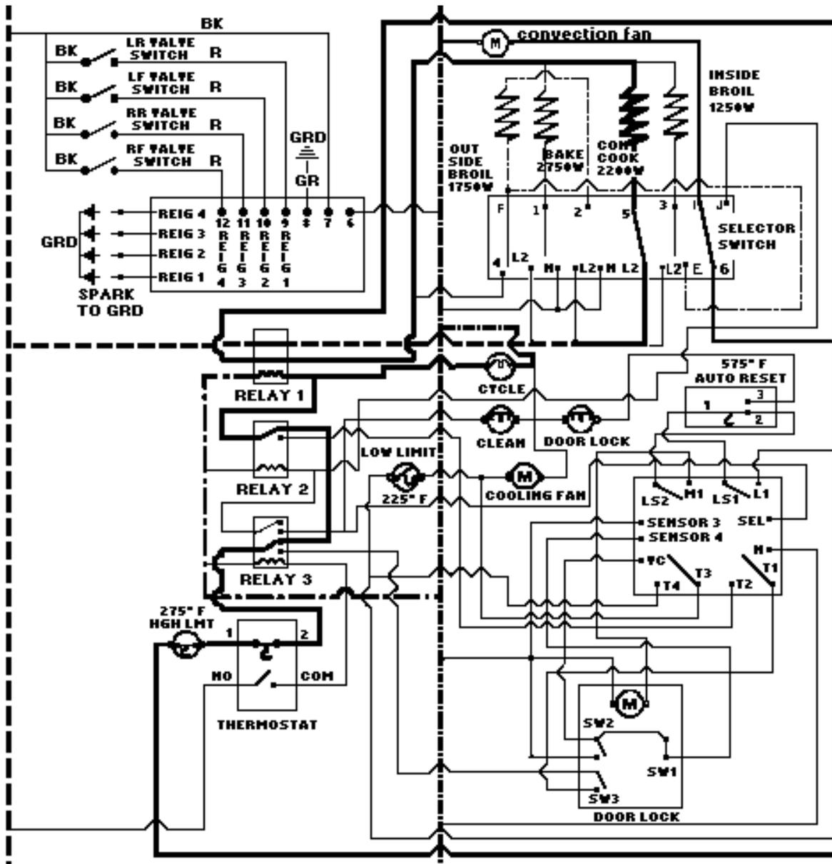
**Selector Convection Cook** position closes Switches 5-L2 and 6-1. 6-1 powers the Convection Fan through L1- at 120v. The Thermostat closes Switch Cy1-Cy2, which cycles with the Oven temperature, powering Relay #1 and the Oven Cycle Light. When Relay #1 closes, it powers the Convection Element at 208v/240v.
