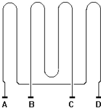
**Broil Element:** "A" to "D" (outside element) 32.6 ohms
