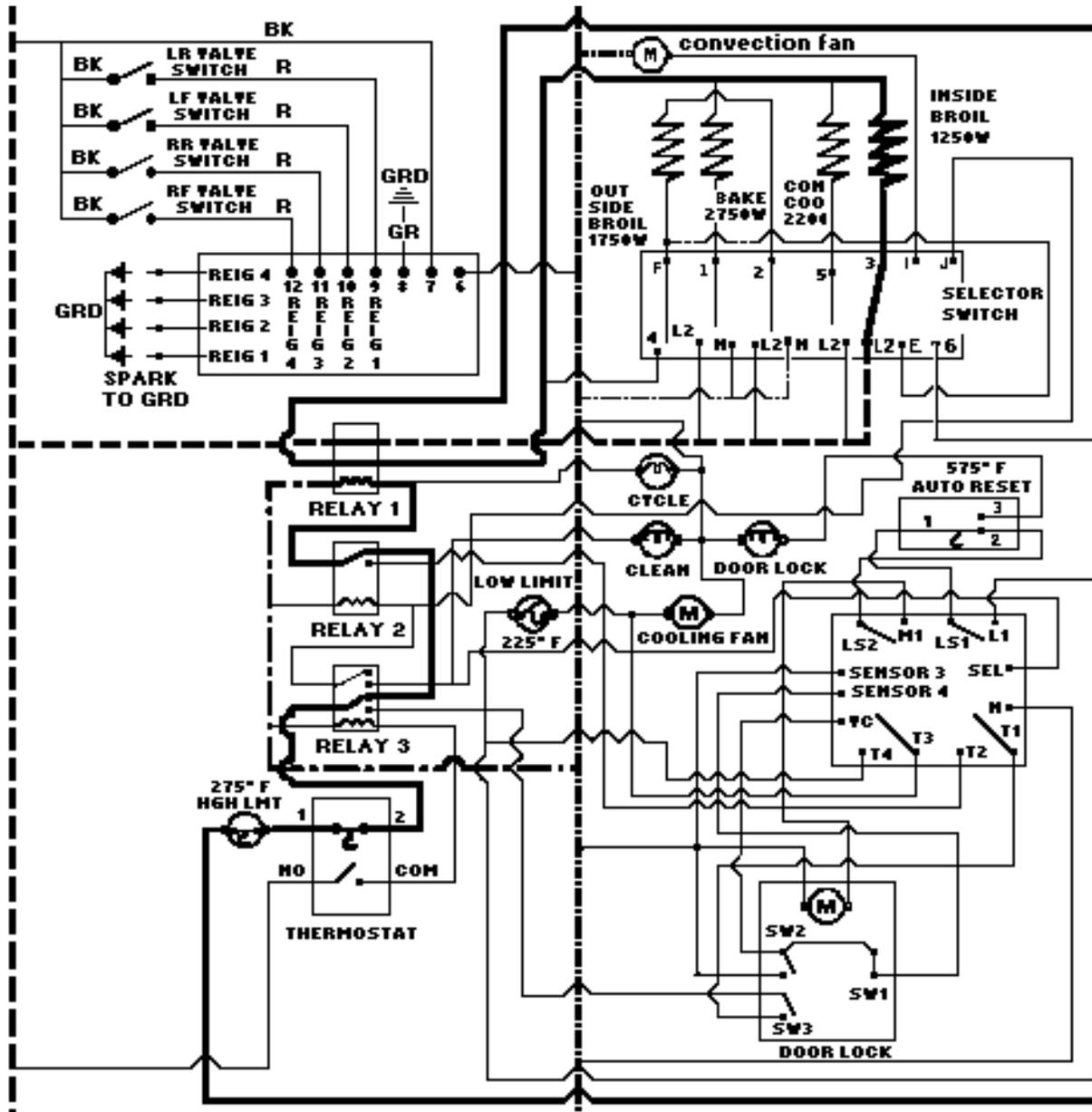
Selector Mini Broil position closes Switches 3-L2. The Thermostat closes Switch Cy1-Cy2, powering Relay #1 and the Oven Cycle Light. When Relay #1 closes, it powers the inside Broil Element at 208v/240v.
