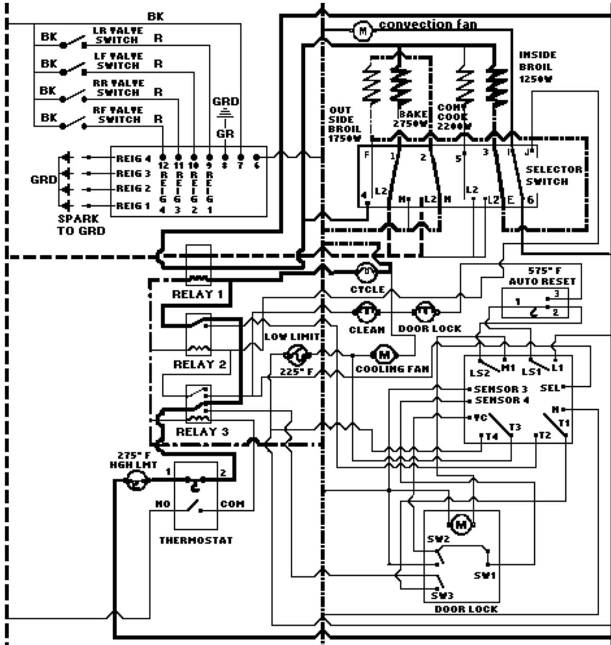
**Selector Convection Bake** position closes Switches 1-L2, 2-N, 3-E, and 6-1. 6-1 powers the Convection Fan through L-1 at 120v. The Thermostat closes Switches Cy1-Cy2, which cycles with the oven temperature powering Relay 1 and the Oven Cycle Light. When Relay 1 closes, it powers the Bake Element at 208v/240v, and with the Broil Element in series across a 120v circuit, it powers the inside Broil Element at 70v and the outside Broil Element at 50v.
