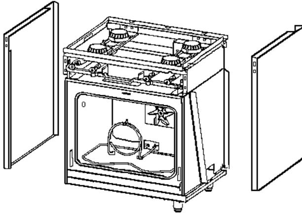
Remove the 6 screws along the upper frame above the door that hold the burner box assembly to the oven body. Lift the front of the burner box high enough to gain access to the **self clean lock** and associated components ( High Limit Switch and Cooling Fan Switch ). Use a block, approximately 6" high, to hold the burner box in place while working on the lock.
