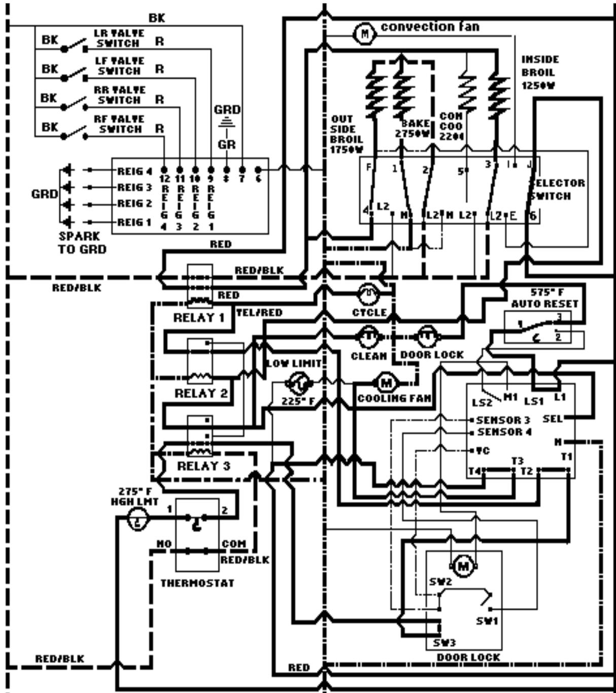
Auto Reset switches to 1-3 which turns Door Lock Indicator Light on and disables Door Lock Motor circuit.
