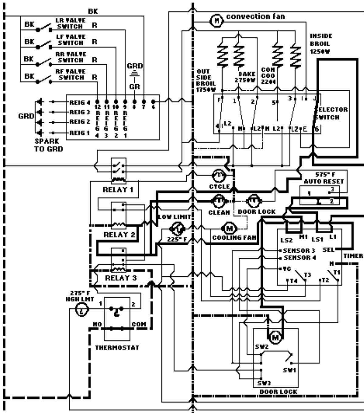
Auto Reset Switches 1-2 closed allowing the Door Lock Motor to operate and turning the Door Lock Light off. The Door Lock Motor operates until 2 seconds after Sensor 4 is signaled by VC that the Door Lock SW1 has been closed mechanically by the Door Lock bolt. The Door Lock / Timer switches LS2-M1 and LS1-L1 open and the Timer resets.
