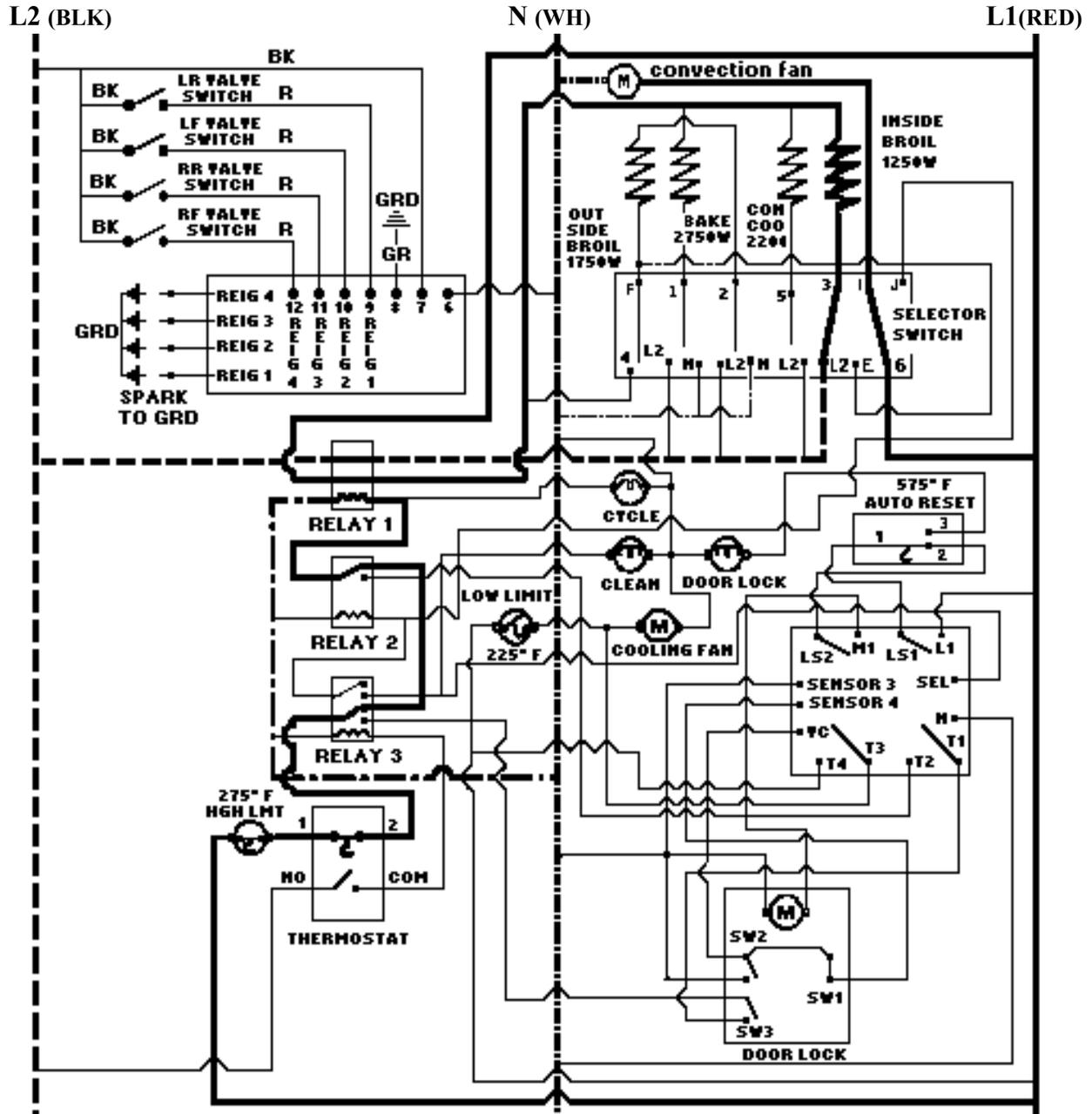
**Selector Convection Broil** position closes Switches 4-F, 2-L2, 3-L2, and 6-1. 6-1 powers the Convection Fan through L1 at 120v. The Thermostat closes Switch Cy1-Cy2, which cycles the Oven temperature, powering Relay #1 and the Oven Cycle Light. When Relay # 2 closes it powers the inside Broil Element at 208v / 240v and the outside Broil Element at 208v / 240v.
