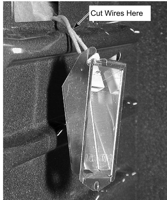
7. Cut the new halogen lamp socket wires to the proper length.
