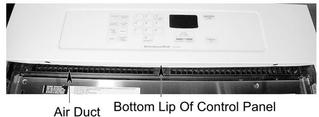
5. Align the mounting holes and install the two side screws in the control panel.
