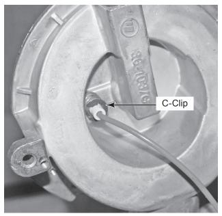
g) Pull igniter and igniter wire out of top of crown burner to remove.
