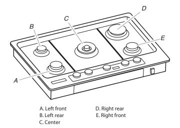
6. Remove all burner caps and burner bases. If necessary, remove the burner ring.
