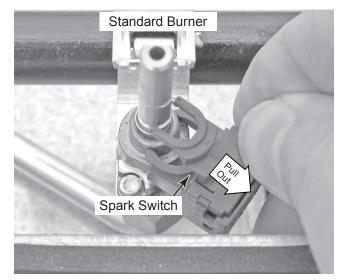
c) To remove the spark switch on the (center) Crown burner, use a small-blade screwdriver, and pry the switch off the valve. **NOTE:** When you reinstall the spark switch on the Crown burner, press down on the spark switch actuator so that it fits under the valve actuator.
