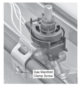
g) Check the rubber seal on the Crown burner gas valve stem and make sure that it is not cracked, or torn. If so, replace the seal.
