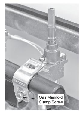
e) Check the rubber seal on the gas valve stem and make sure that it is not cracked, or torn. If so, replace the seal.
