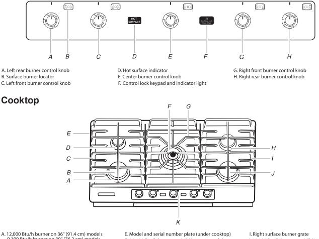
A. 12,000 Btu/h burner on 36" (91.4 cm) models 9,100 Btu/h burner on 30" (76.2 cm) models B. Surface burner cap
