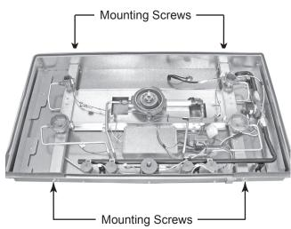
f) Lift burner assembly out of burner box.
