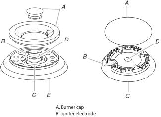
B. Igniter electrode C. Burner base D. Gas tube opening E. Burner ring 6. Using a T20 TORX® screwdriver, remove the orifice holder screws (C).
