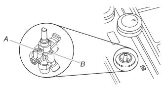
A. Adjustment screw - inner crown B. Adjustment screw - outer crown
