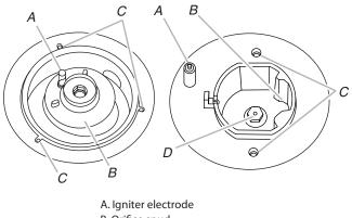
B. Orifice spud C. Orifice holder screws D. Orifice holder
