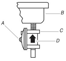
A. Access cap B. Rear of cooktop C. Gas pressure regulator D. Gas flow
