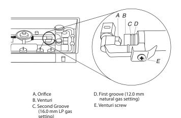
• Use 15.0 mm wrench to loosen the nut securing the tube to the orifice pack. Remove the tube from the orifice pack.
