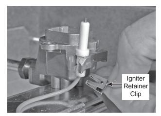
c) Remove igniter from standard burner.
