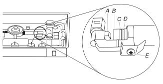
A. Orifice B. Venturi C. Second Groove (16.0 mm LP gas setting)
