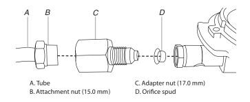
• Use 17.0 mm wrench to loosen and remove the orifice pack.
