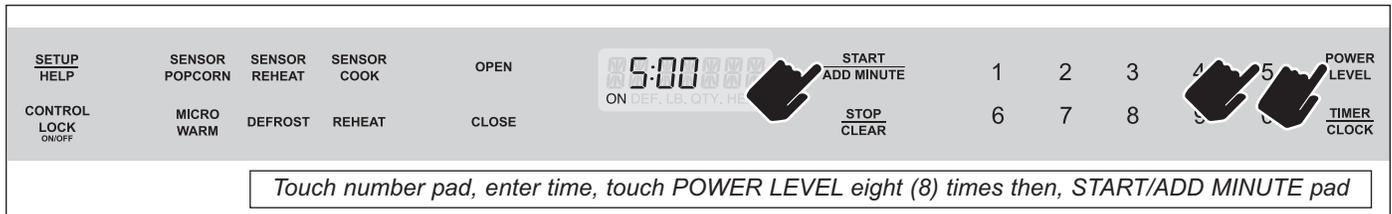
Figure 3-8. Setting the POWER LEVEL
