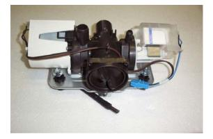
The recirculation pump is separate from the drain pump, but they are attached to opposite sides of the filter housing.
