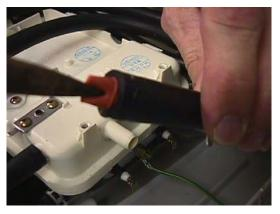
Be particularly careful when removing and replacing the water input hose to the steam generator. There is a check valve that fits into the input port. The valve sometimes comes off and is stuck in the hose. This could cause the water not to flow, which would cause the steam generator to malfunction.
