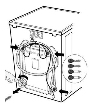
The wrench, shipping bolt hole covers, drain hose tie-down strap, and a sample packet of detergent are included in a packet shipped inside the washer.
