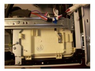
The steam generator has two water connections: water in and steam out. The water is supplied by one of the solenoids on the cold water input. The steam from the generator is directed through a rubber hose to a nozzle at the top of the door gasket, where it sprays out through the laundry as it tumbles.
