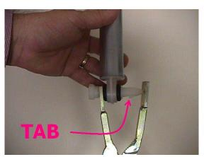
Use special tool **383EER4003A** to remove the damper pins. If you are replacing the dampers, you'll have to remove both ends. If you are removing the tub for major repair work, disconnect the damper ends at the base and leave the other ends connected until you remove the tub. When putting the tub back into the machine, connect the dampers to the tub first. It is much easier that way.
