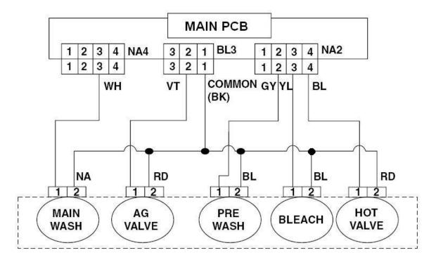
The solenoids can be checked in TEST MODE. (See page 52.) Use a multimeter to verify that each solenoid is receiving 120  $V_{AC}$  during the TEST MODE. Also verify that the proper valve is dispensing water to the appropriate dispenser compartment. This procedure can also be used to determine that the valves are connected correctly and the hoses are routed to the appropriate compartments after a repair.
