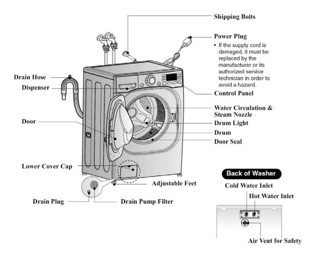
The air vent on the back of the machine must be left open and clear at all times.
