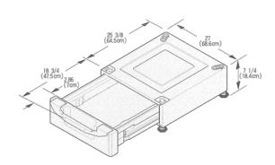
Remove the pedestal, installation hardware, and instructions from the shipping carton. Set the pedestal as close to the installation position as possible.
