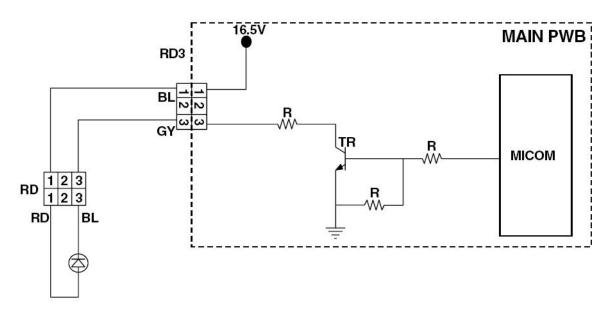
Testing between pin 1 or pin 3 and chassis ground at the lamp connector when the lamp should read approximately 16.5  $V_{DC}$  whether the lamp is on of off. When the microprocessor switches the lamp on, the current is passed to ground through a resistor, effectively dropping the voltage at the lamp to 6.5  $V_{DC}$ .
