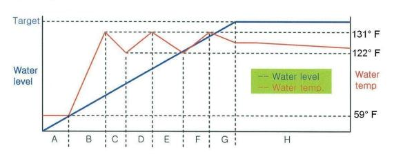
In example 2, HOT / COLD temperatures are chosen for a NORMAL cycle. The prewash valve is opened and cold water is supplied briefly, then the hot valve is opened and water fills the tub to the target water level. This water never reaches the set point, so the heater is energized. When the water temperature reaches 122° F, the heater is turned off.
