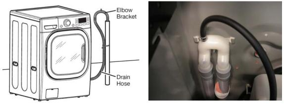
The drain pipe should be firmly attached to the standpipe or the laundry tub or sink where it drains. The pump has sufficient power to cause the pipe to move around when the water is expelled. The pump can lift the drain water a maximum of 96 inches (2.4 m), but there is no minimum height requirement. The vacuum breaker in the drain line will prevent drainage by gravity or siphoning. The hose can lay flat into a floor drain as long as the end of it is not submerged.
