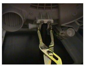
The flat end of the tool goes on the small end and the split end allows the head end to pass through while the pin is pushed out. Sometimes you can use a socket to hold the pin down while you press the pin out.
