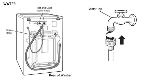
Be sure the rubber washer is inside the hose end. Attach the hoses to the washer (red is HOT, blue is COLD). Tighten them firmly but don't strip the plastic threads on the washer connections. The hoses are clearly marked by temperature. The HOT hose is thicker and has a higher temperature rating and burst strength.
