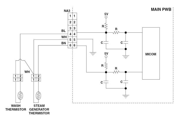
Use an ohmmeter to check the resistance of the sensor when it is disconnected from the circuit.
