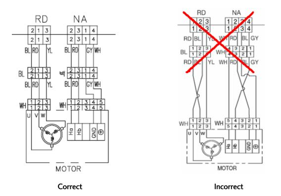
Pay particular attention to the **color codes** and the **position numbers** in the connectors. This will be critical when you take voltage readings to determine component malfunction. Hall Sensor testing methods are now available on the following pages when LE error code troubleshooting says "*hall sensor is out of order or defective.*"
