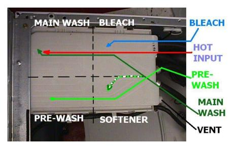
The dispenser works by using various solenoids to apply water to different compartments. The liquid products are dispensed from a siphon box. As the appropriate chamber is flooded, the box fills and the water flushes the laundry product into the tub. It is mixed with water before contacting the laundry to prevent spotting or damaging the fabric.
