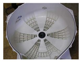
Unbolt the bolts around the circumference of the seam. (top photo) Separate the halves. Be careful to avoid damaging the gasket. Do not pry on the surfaces between the halves.
