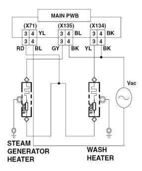
When using the connectors for test points, pay particular attention to connector and wire colors and numbers.
