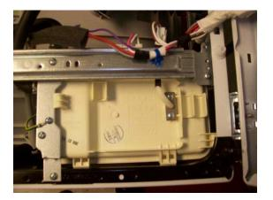
Push the steam generator toward the back of the washer to release it from the side rail. You can then remove it for draining, inspection, and replacement.
