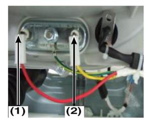
The wash heater is at the bottom of the tub where it heats the water in the sump.
