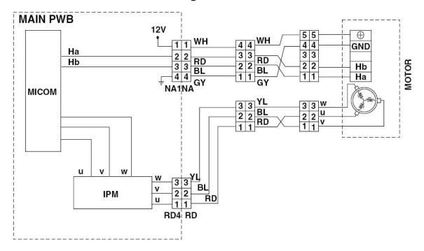
The stator can be tested either from its connector or from the connector at the main board. Either one must be disconnected before reading the resistance with an ohmmeter.
