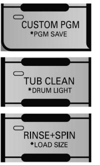
When the user inputs a custom program, press and hold CUSTOM PGM for three seconds until it beeps twice. Thereafter, this button will run that custom program.
