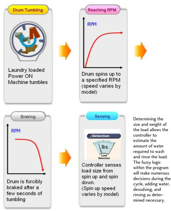
At the beginning of the cycle, the washer tumbles the load to determine its weight (see previous page) and displays the approximate load size via the LOAD SIZE ICON. The measurement suggested on the icon will allow you to adjust the amounts of detergent, bleach, and softener for improved economy and efficiency.
