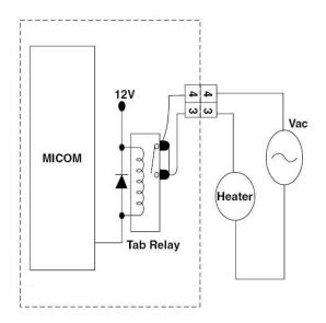
When the heater is energized, use your multimeter to read the voltage. It should be approximately  $120 V_{AC}$ .
