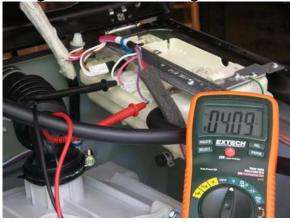
The photo to the left shows the high water sensor (VIOLET) wire. As the caption shows the meter is reading a voltage of  $4.09 V_{DC}$ . Water in the housing is not touching the high water probe. When this occurs, the control board would activate the cold inlet valve for the steam generator before energizing the heater, IF steam was selected and the control board wanted steam.
