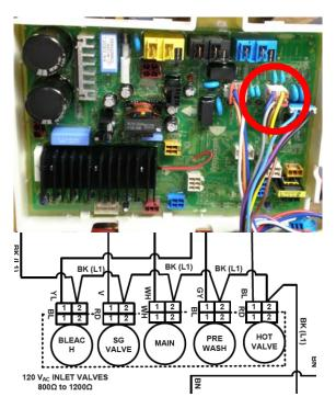
At this connector on the main board, all four wires are the neutral side of the line. Voltage is applied to the solenoids by the BLACK wire and the neutral side is completed or broken to actuate each solenoid.
