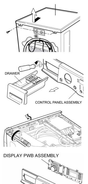
Remove the screws securing the top plate (cover.)
