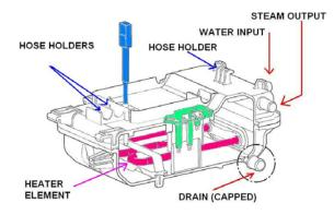
The steam generator can be removed as an assembly for diagnosis and replacement or tested in place.
