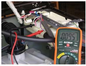
In this picture we see the meter displaying less than 1.5  $V_{DC}$ . In this example, the water in the housing is touching the high water sensor probe and the ground probe. When this occurs, conductivity through the water is measured as a voltage drop and the control board knows the water housing is full of water.
