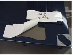
Depending upon the model, your pedestal may have straight or curved brackets. The curved ones are to be used on the rear positions when mounting a dryer to a pedestal, but can also be used in any other position on the pedestal.
